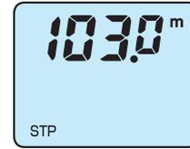
1. Press **MODE BUTTON** six times to show on the display real fishing time and total winding length.
